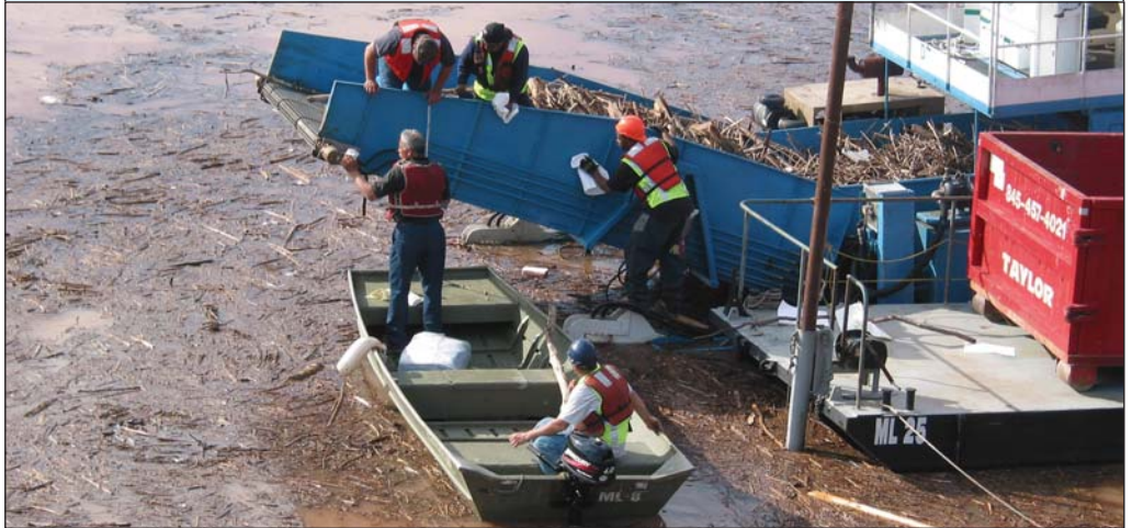
A BWT Skimmer Boat Assists in Capturing Debris in the Ashokan Reservoir
