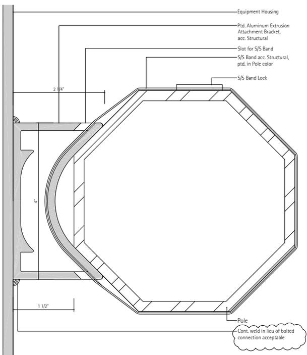
2 Plan Section through pole at Box Attachment Bolt
