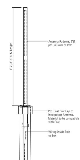
3 Alternative Double Antenna Scheme, Wishbone, Elevation
