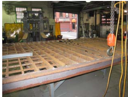
New Grizzly Under Fabrication for the Agency Asphalt Plant. (Credit: Russell Holcomb)
